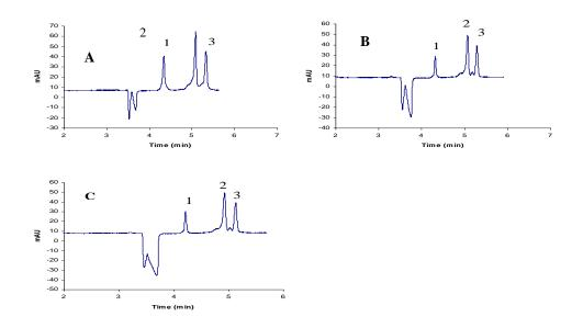
A) Sample without plug, B) Injection of undiluted plug of BGE behind the sample and C) Injection of a 100 times diluted plug of BGE in front of the sample. Condition: 50  $\mu$ m i.d. capillary, BGE; NH<sub>4</sub>Ac at pH 4.0, 70 mM, field strength: 310 V/cm, protein samples dissolved in 10 times diluted BGE (0.1 mg/mL) and injected at 50 mbar for 6 sec. The amount of sample injected was 0.95 ng. Sample: 1)  $\alpha$ -chymotrypsinogen A, 2) lysozyme and 3) cytochrome c.
